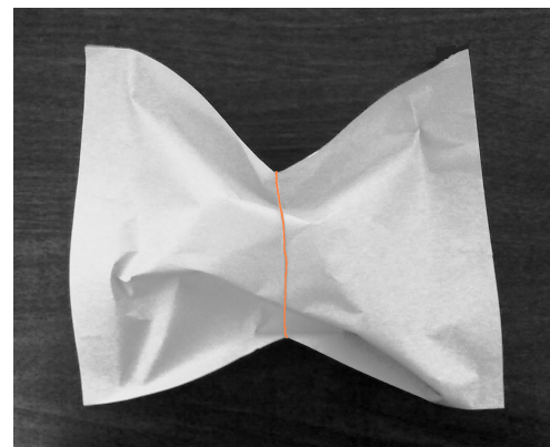
Fig 6 - The distortion of a butt-welded plate, illustrated by putting a rubber band on a sheet of paper
